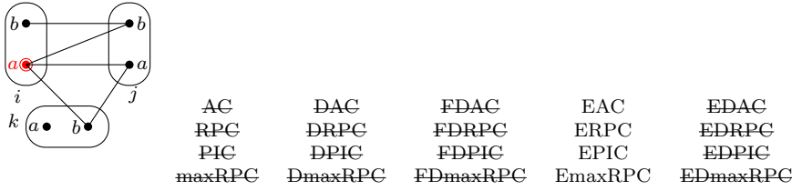
Fig. 11 A WCSP which is existential consistent but is full directional inconsistent. i > j > k . The problem is not AC (hence is not RPC, PIC, maxRPC) because of value (i, a) (has no arc support in c_{ij} ) and is not DAC (hence is not DRPC, DPIC, DmaxRPC) because of value (j, b) (has no full arc support in c_{ij} ). However, the problem is EmaxRPC (hence EPIC, ERPC, EAC) where (i, b), (j, a), (k, a) are respectively EmaxRPC supports of i, j, k .
