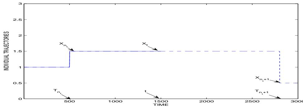
$\Delta T_{n+1} = T_{n+1} - T_n$  (waiting time between 2 jumps)
